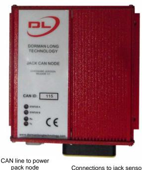
Connections to jack sensors and hydraulic valves
