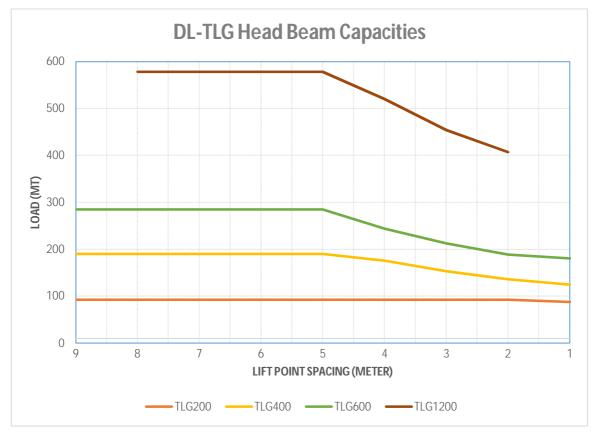
The above graph is plotted considering maximum span = 11.3m, Load centre offset = 0m and  $1^{st}$  stage of the ram. For complete lifting arrangement and duty charts please refer the respective telescopic lifting gantry drawing.
