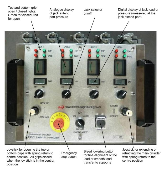
The wiring and junction boxes on the jacks and power packs are the same for both the DL-P40 and DL-M systems, allowing the DL-M system to be used as a back up to the DL-P40 computer control system with a very quick changeover form one system to the other.
