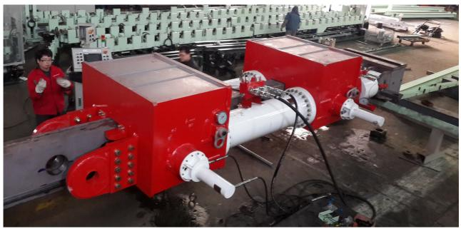
DL-CP600 pinned climbing jack load testing
