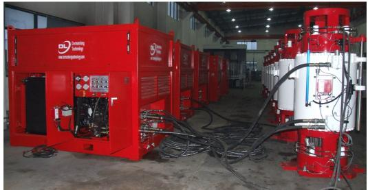
DL-L120/2/300/D Diesel powered hydraulic power packs
