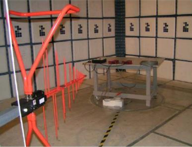
Radiated Emission Test Set-up Back View
