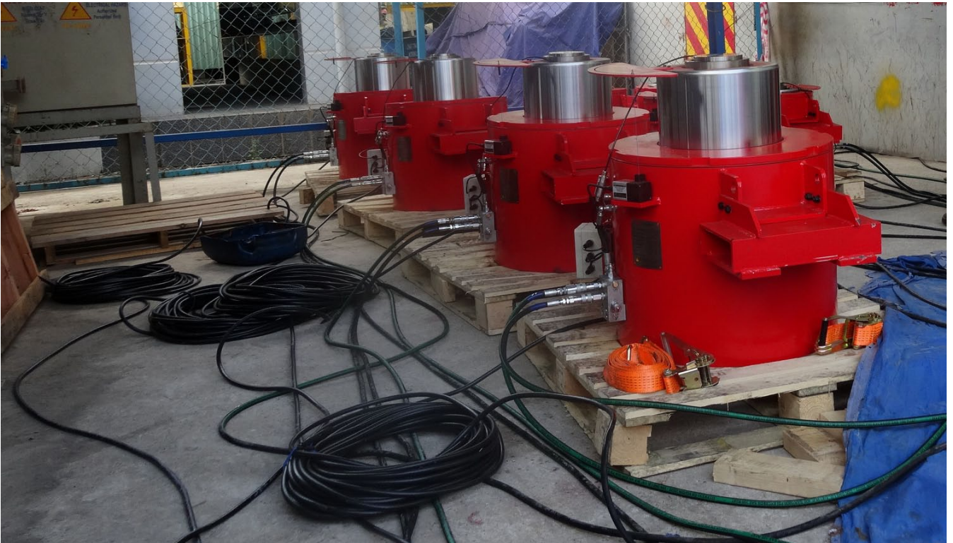
4 No DL-WJ600 weighing jacks with load cells of 0.5% load accuracy. 200mm stroke, 600 MT SWL per jack.
